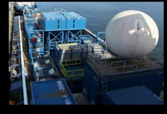
During October and November, Baker Hughes assembled a frac plant on the main deck of the MV Art Carlson in Luba, Equatorial Guinea. An oil or gas well is frac'd by pumping tons of small ceramic balls (proppant) under high pressure to open up the reservoir for better drainage and higher flow rates. The proppant keeps the fracture "propped" open.
