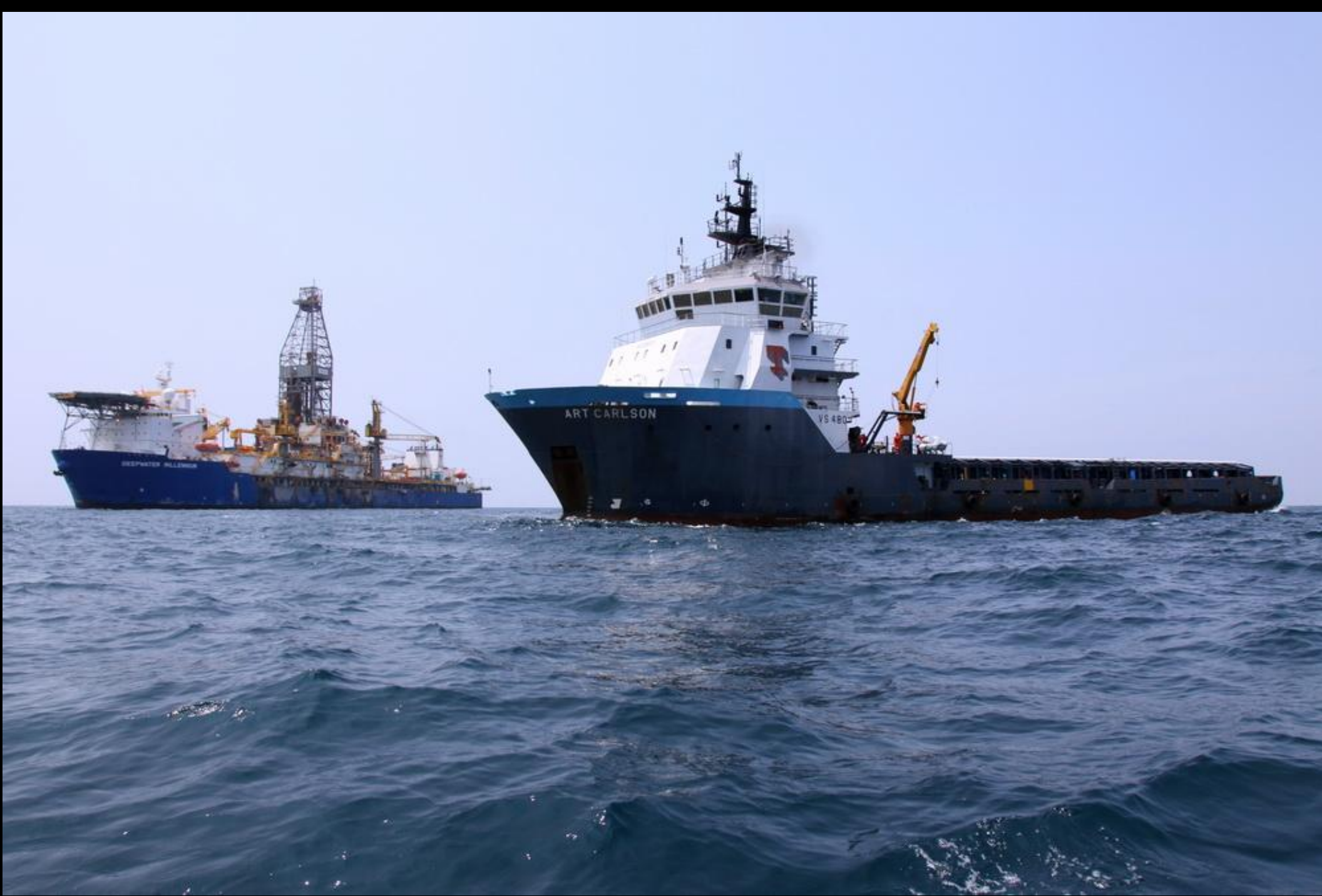
She has two deck cranes rated at 20,530 pounds each at 33 feet reach.
