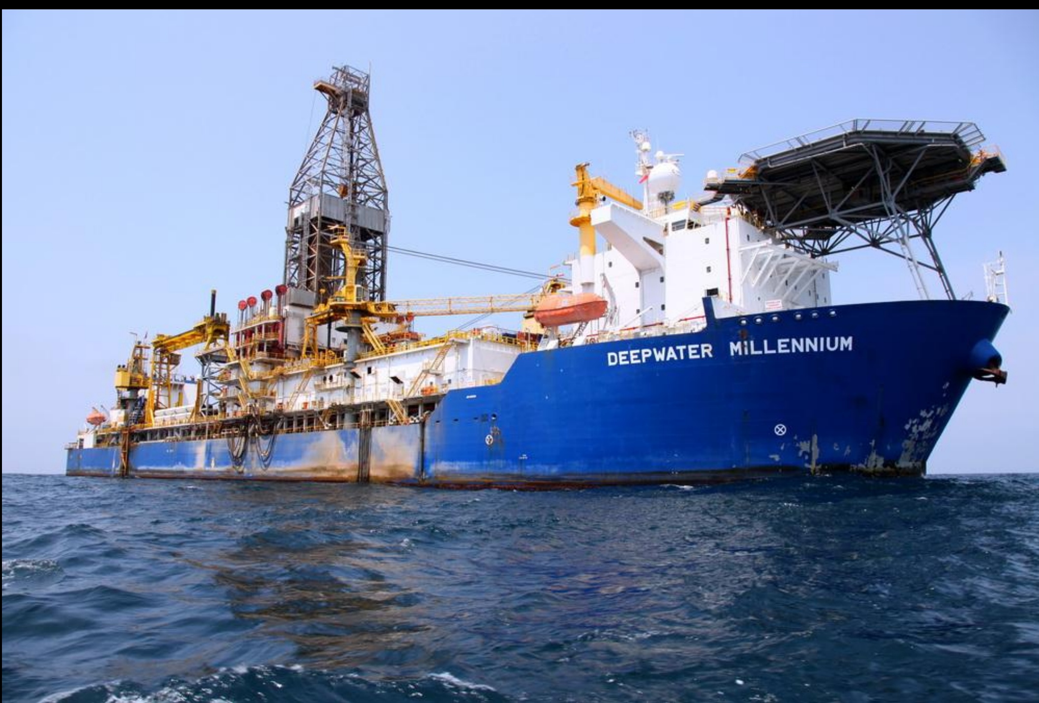
Her function here in Ghana is to complete and test some of the gas wells in the Tano Field.
